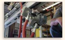
We have added color-coded tags to make connecting the pneumatic hoses an easier task.
