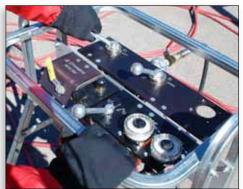
The **Control Box** operates the lancing system and positioner air motors. It is simple to set up, operate and move about. An air filter and lubricator are included for air motor maintenance. 25 ft of 1/2" air hose is supplied for each air motor.
